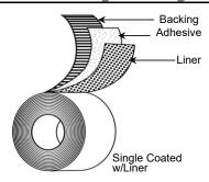
**Backing:** Exterior-Grade Aliphatic Polyurethane
